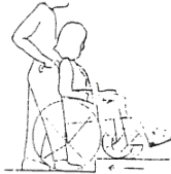
Figure 4. When the wheelchair is being rolled backwards off a curb, support it by lightly pressing against it.
